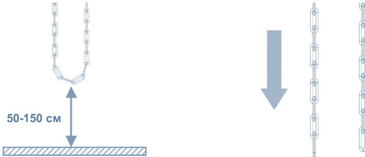
Fig. 6. Door control with chain reducer
